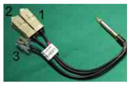
Figure 3. Probe for the measurement of intramedullary perfusion and temperature near the bone cortex, with metal reinforcement in the rear area and the jacks for connection with the laser Doppler and temperature units. 1: Afferent optical fibre cable, jack. 2: Efferent optical fibre cable, jack. 3: Cable for temperature measurement, jack.
