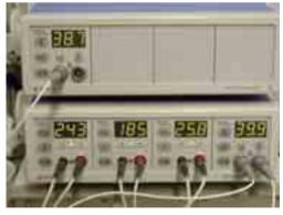
**Figure 6.** Three laser Doppler PF5010 LDPM units and two PF5020 temperature units (Perimed, Sweden). Each temperature unit contains two temperature measurement channels.
