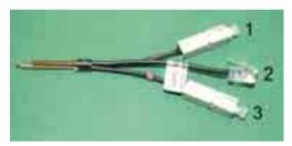
**Figure 1.** Probe made entirely of PSU for the measurement of intramedullary perfusion and temperature near the cortex, with integrated afferent and efferent optical fibre cables and cable for the temperature sensor, and the jacks for connection with the laser Doppler and temperature measurement units. 1: Efferent optical fibre cable, jack. 2: Cable for temperature measurement, jack. 3: Afferent optical fibre cable, jack.
