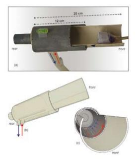
Figure 2. (a) Dorsal view of apparatus to prevent heat loss in anaesthetized gerbils. (b) Schematic ventral view of apparatus. (c) Schematic frontal view of apparatus. Arrows indicate water of 38 °C flowing between the two tubes (red: inflowing, blue: outflowing).
