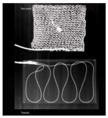
**Figure 3.** Radiograph of the used homeothermic blanket (N-HB101-S-402, Panlab, Barcelona, Spain) (below) and Harvard blanket (Harvard Apparatus , Massachusetts, USA) (above)
