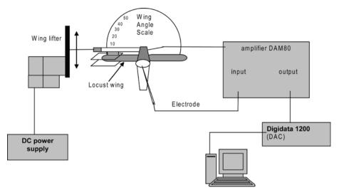
Figure 1. Experimental setup for recording activity from locust wing stretch receptor.
