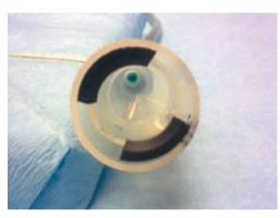
Figure 4. Rubber gasket.
