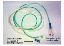
Figure 5. The LCF mask with the breathing system.
